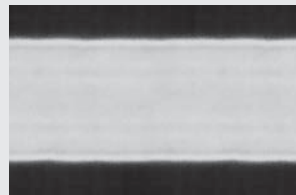
Latex paint through a standard 517 tip at 1,000 psi
